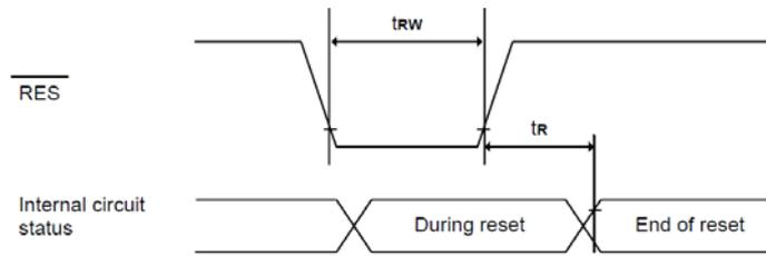
( $V_{DD} - GND = 1.65V$  to  $3.5V$ ,  $T_a = 25^\circ C$ )
